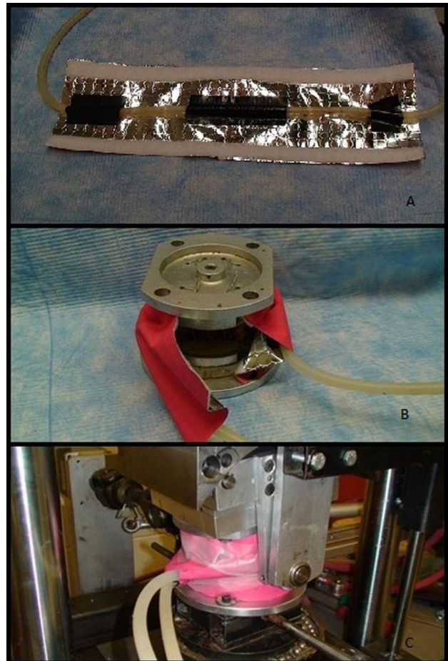
Fig. 1 (a) Heating jacket used to bring the specimens to sufficient temperature for the hydrogel to change from a liquid to a gel state. Rubber tubing was attached circumferentially and had heated water cycled through it. (b) The jacket itself was then wrapped around the metal cups used to secure the specimens. This ensured that the heating jacket was not in physical contact with the specimen and did not interfere with the flexion or extension motions of the segment while still providing heat. (c) Entire heating jacket configuration secured around the specimen while being cyclically fatigued.
