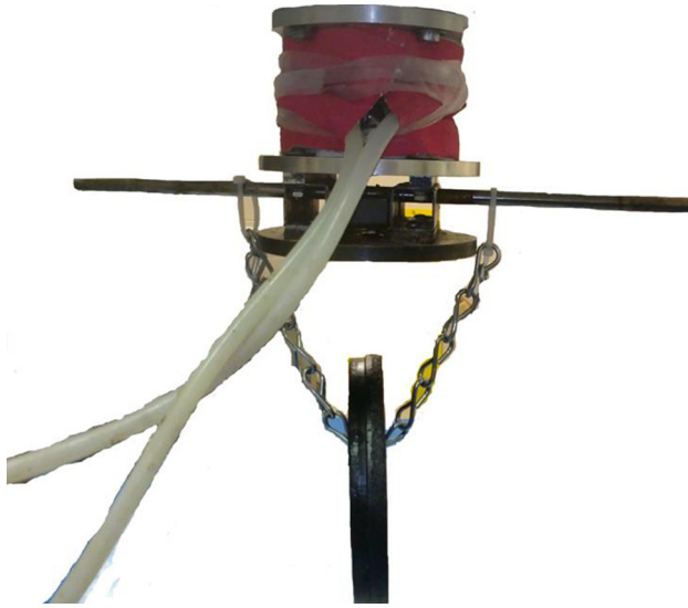
Fig. 2 Custom-built apparatus used to provide traction to specimens in order to achieve sufficient endplate separation facilitating hydrogel injection. Specimens were suspended while a 5 kg weight was hung to the carriage holding the bottom disc in place. A sleeve with tubing running heated water on its periphery provided heat to the specimens without interfering with flexion or extension motions.
