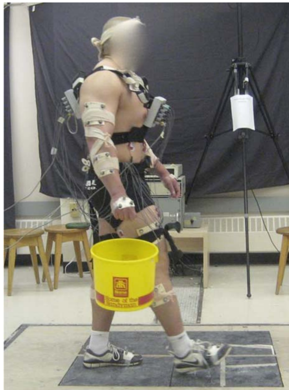
Figure 1. Photo of subject carrying buckets either in one hand or with two hands while striding onto force plates. EMG is recorded for the torso musculature, together with 3D body segment kinematics.
