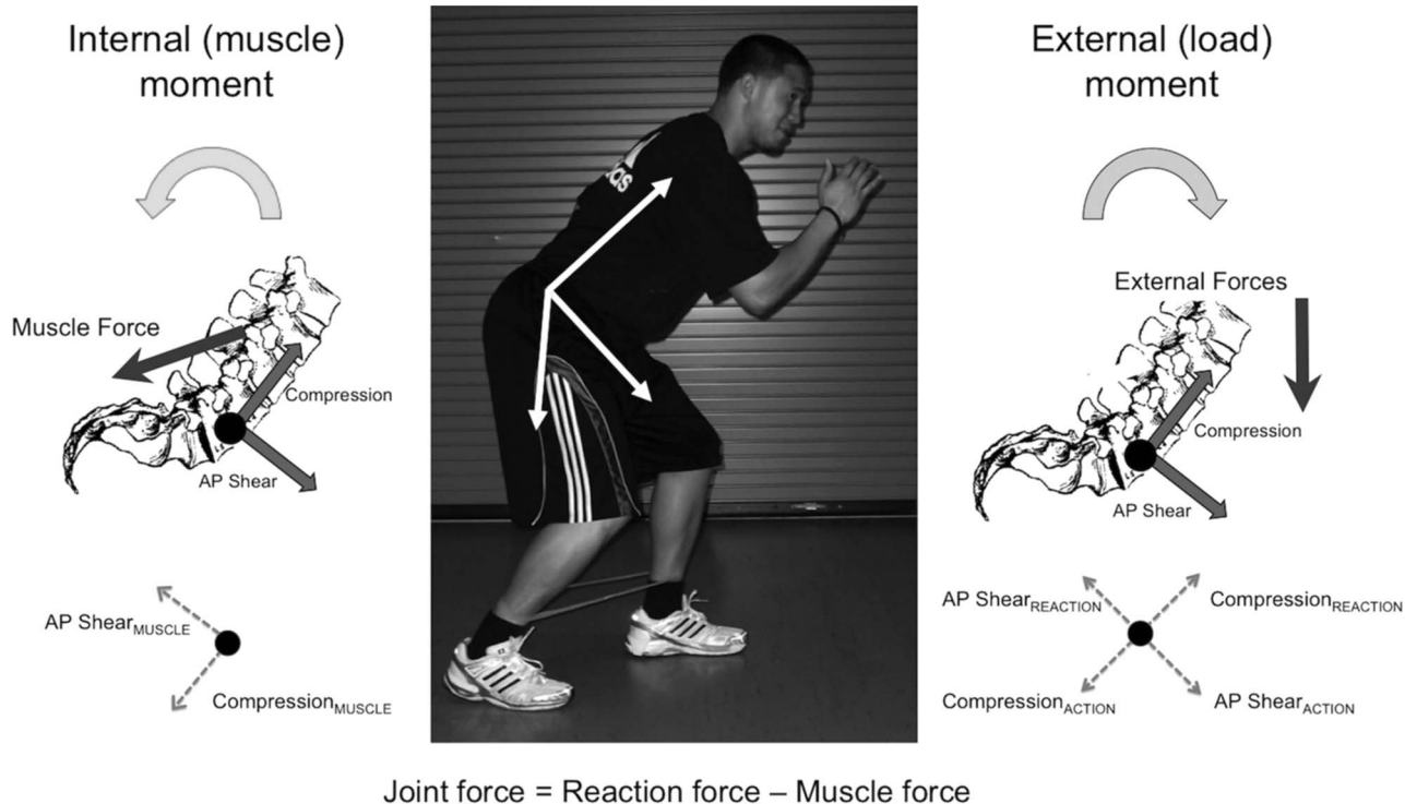
Figure 2. The internal (muscle) and external (load) moment were computed with the processed EMG and lumbar spine motion, and video and hand forces, respectively. The L4/L5 joint (i.e. bone on bone) force (compression and shear) was calculated by subtracting the muscle force from the reaction force.
