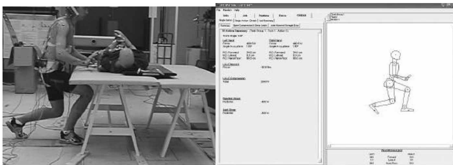
Figure 4. Kinematic posture obtained from video data and corresponding posture with 4D Watbak model. The Watbak analysis shows output of L4-L5 moment, compression and joint shear.
